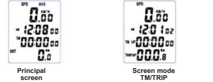
General data and Data of time and distance traveled by pedaling (UP) and without pedaling (DN)
